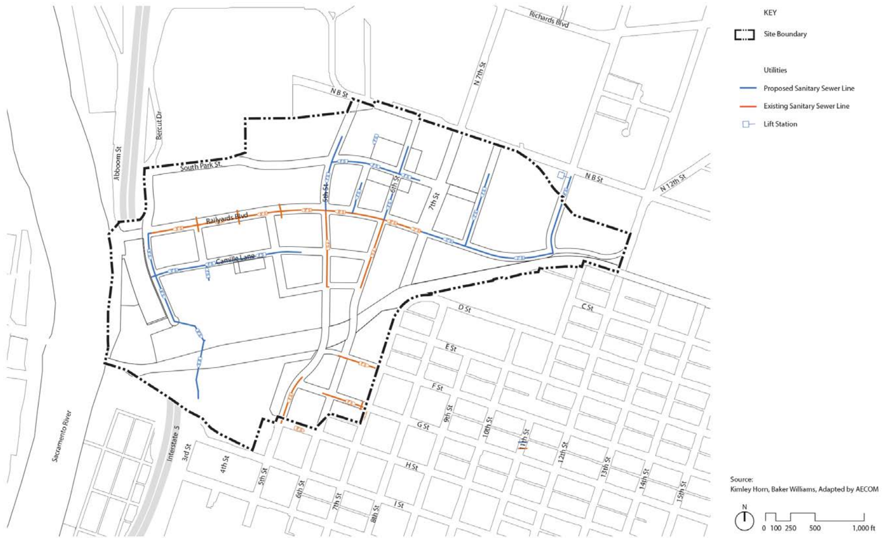
Figure 7-2. Conceptual Sanitary Sewer System
